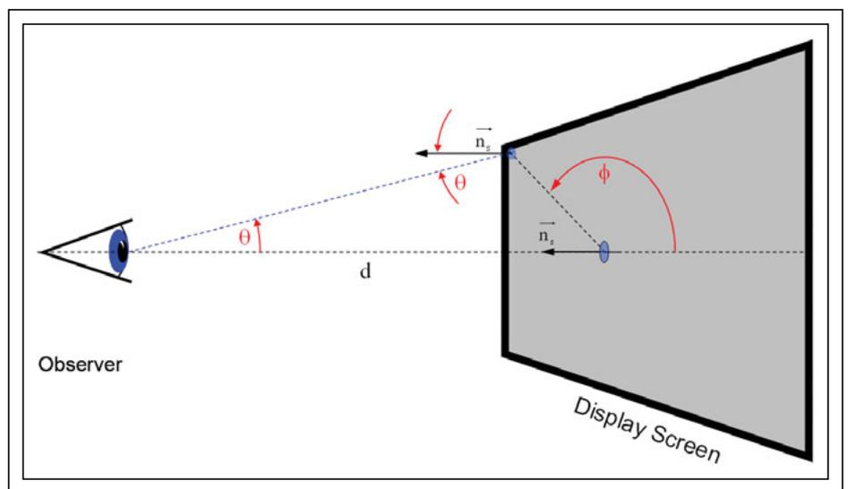
**Fig. 1:** The observer looks at every location on the display screen from a specific direction (viewing direction) specified by the spherical angles,  $\theta$  (angle of inclination) and  $\phi$  (azimuth).
