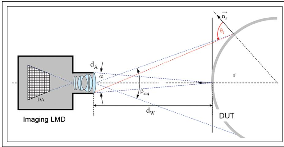
**Fig. 6:** Here, an imaging LMD is applied for the evaluation of, e.g., the luminance of a cylindrical DUT. With the measurement field angle,  $\beta_{img}$ , up to 40° (typical 20°), the variation of the angle of inclination across the DUT is more pronounced and thus affects the results. In addition, the area element at the periphery of the measurement field is more distant from the lens than the on-axis area element and thus defocusing takes place.
