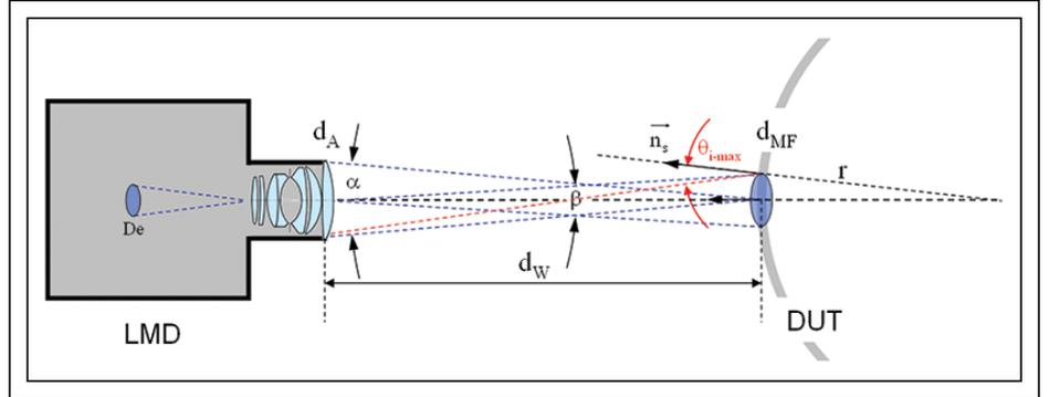
**Fig. 5:** The angle of inclination ( $\theta_i$ ) at the periphery of the measurement field (MF) with respect to the local surface normal ( $\vec{n}$ ) is given by the diameter of the objective lens aperture ( $d_A$ ), the distance between the lens and the measurement field ( $d_W$ ), the diameter of the measurement field ( $d_{MF}$ ), and the radius of the cylindrical DUT,  $r$ .
