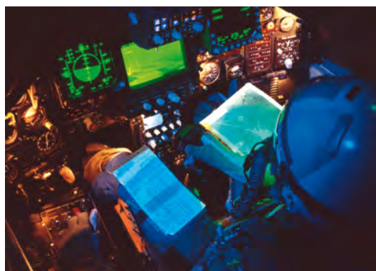
Fig. 3: DTS 140D NVIS allows MIL-L85762A / MIL-STD-3009 compliant measurement of night vision displays and panels (e.g. in aircraft cockpit).
