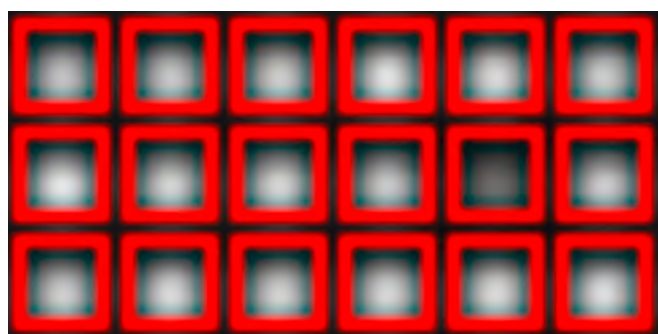
▲ Figure 3: Zoom into detected \mu OLEDs. The red squares represent the detected grid of emitters, indicating that the horizontal and vertical pitch is identical. The white dots in the cells are the emitters.
