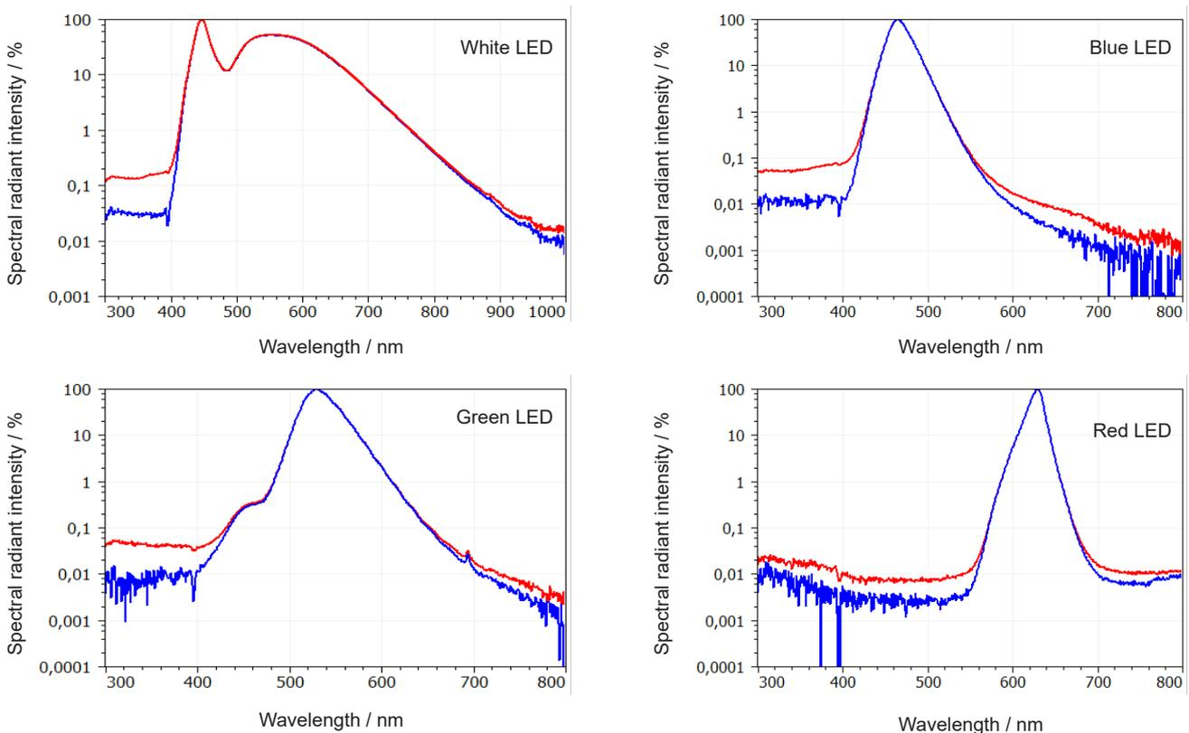
Fig. 6: Logarithmic display of the spectra of white, blue, green and red LED without (red) and with stray light correction (blue).
