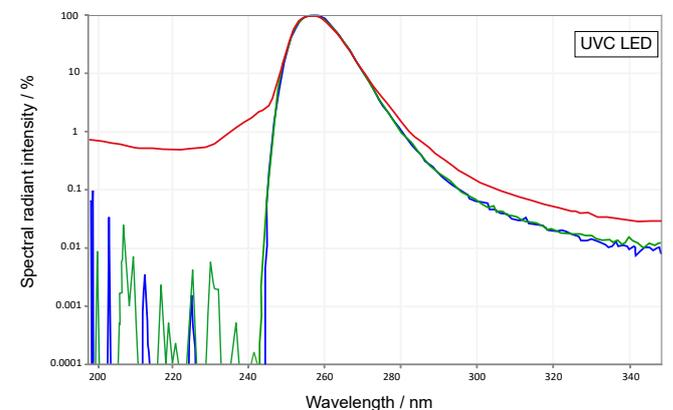
Fig. 5: Logarithmic display of the spectra of a UVC LED without (red) and with stray light correction (blue) and measured with a double monochromator (green).
