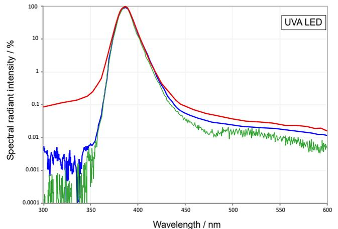
Fig. 4: Logarithmic display of the spectra of a UVA LED without (red) and with stray light correction (blue) and measured with a double monochromator (green).
