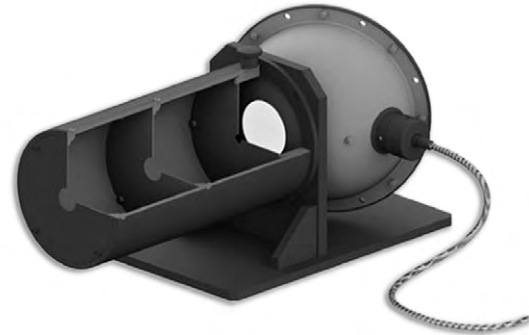
Figure 3: Implementation of the alternative method with the PTFE integrating sphere and a tube with all the necessary apertures for BLH measurements.
