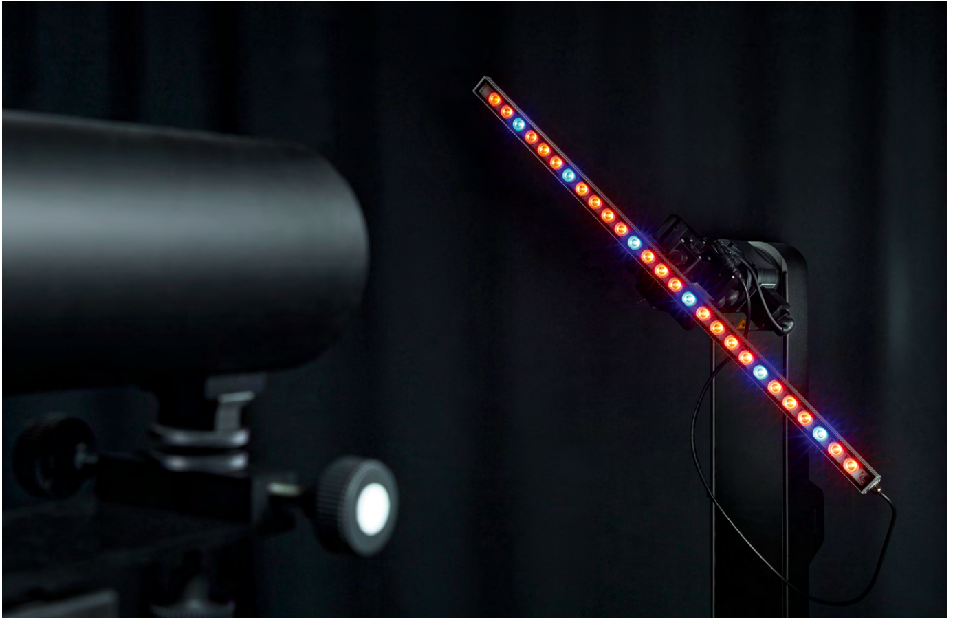
Figure 4: Turning luminaire with a detector tube. Insufficient extraneous light suppression is a typical source of error in the measurement lab.
