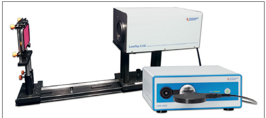
Figure 1. Ultra-high resolution 2D imaging colorimeter with spectroradiometer in a laboratory setup.
