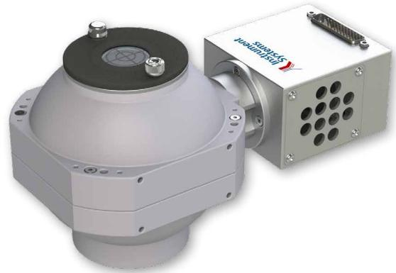
The ACS 585 LED luminance standard from Instrument Systems GmbH is a highly stable light source based on LED technology. Its light is homogenized by an integrating sphere. The ACS 585 is used to verify absolute measuring accuracy of the luminance meters. Instrument Systems provides accredited testing service for luminance.
