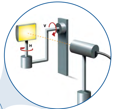
Direction of rotation of a Type A goniometer.
