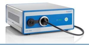
The high resolution CAS 140D-HR is based on Instrument Systems' well-proven high-end array spectroradiometer CAS 140D. Particularly designed for the measurement of narrow band emitters, e.g. laser diodes, the CAS 140D-HR combines high spectral resolution and short testing times for sophisticated production and laboratory applications.
