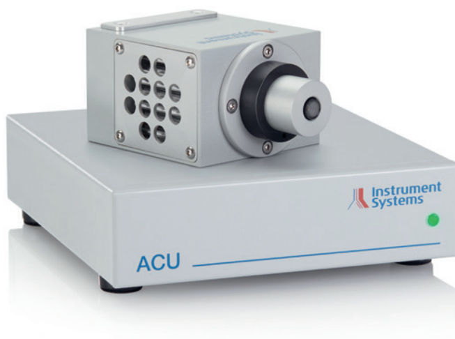
The ACU is a compact control unit for ACS calibration standards containing a high-precision constant current source and a TEC controller for accurate temperature stabilization. The ACU has been developed for both laboratory and production use.
