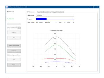
DMSOcto app, showing measurement progress and luminance vs. angle graph.
