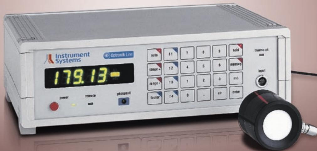
The Digilux 9500 is a precision luxmeter that enables convenient measurement of illuminance in a laboratory or on the production floor.
