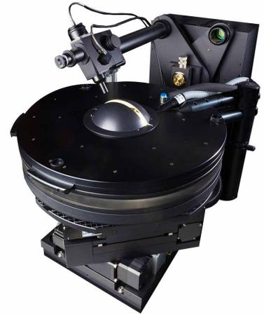
The HCS-3B is an optional mechanical component for the DMS 803, DMS 505 and DMS 201 display measurement systems. This heat-cool system – available in different variants – enables temperature-dependent measurements of optical display properties and conformance testing. It is used to measure electro-optical and switching characteristics under arbitrary directions of observation as well as angular scans over the viewing cone.
