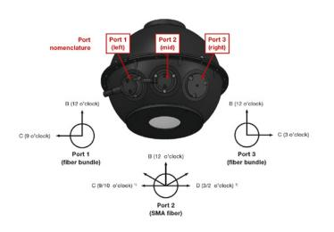
The fiber bundle and SMA adapters can be oriented either perpendicular (12 o'clock position) or parallel (9 or 3 o'clock) to the measuring plane as displayed above. For the ISP 250-PTFE SMA adapter, 10 and 2 o'clock are available in addition to the perpendicular orientation (12 o'clock).
