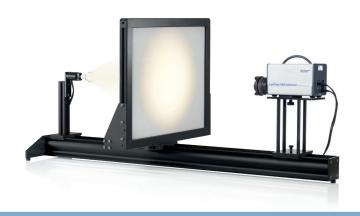
The LVK analysis kit is the perfect add-on for a quick and precise determination of luminous intensity distribution curves with the LumiCam imaging colorimeter. It consists of an optical bench (length 2 m), an opaque screen (effective width 610 mm, effective height 480 mm) and riders to accommodate LumiCam and light source.
