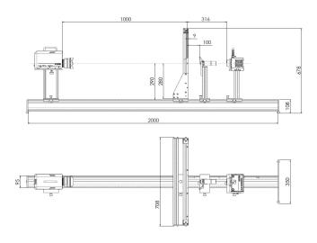
The LVK analysis kit for the measurement of luminous intensity distribution curves, complete with a bench, an opaque screen, a carrier for a LumiCam, a carrier for a light source, a light source and a laser with a carrier.
