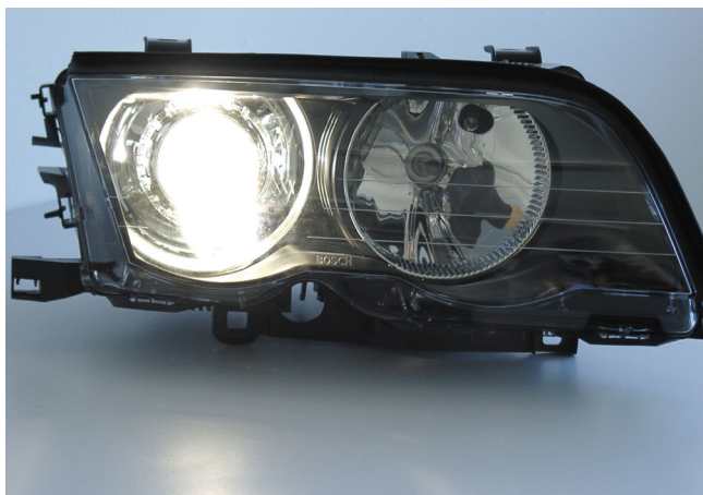
HID (Xenon) Headlamp operated by SNT 10
