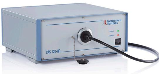
▲ The spectrum of each single emitter can be measured with CAS high-resolution spectrometers
