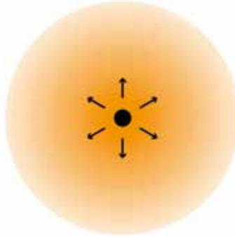
Light is electromagnetic radiation and thus a kind of energy. Radiant power  $\Phi_e$  is defined as the energy  $dQ_e$  of optical radiation emitted by a source per unit time  $dt$ . The unit of radiant power is the watt [W].
