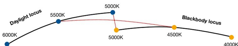
The main result of a TM-30 calculation is the Fidelity Index  $R_f$  and the Gamut Index  $R_g$ .  $R_f$  scores from 0 to 100 and can be interpreted as a more accurate version of CRI<sup>8</sup>. The value set of the Gamut Index depends on the achieved Fidelity Index. It scores from 60 to 140 when  $R_f > 60$ .  $R_g < 100$  means decreasing overall saturation and  $R_g > 100$  means increasing overall saturation.
