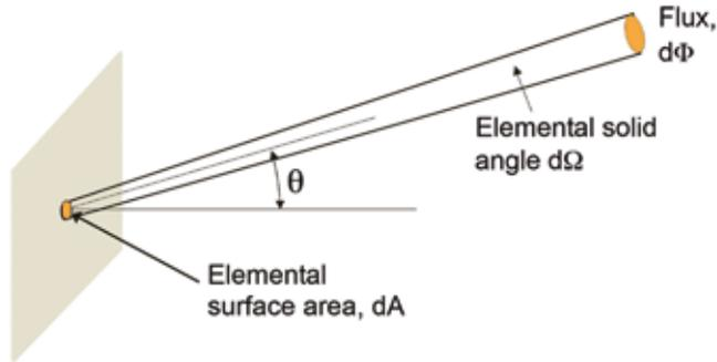
Radiance  $L_e$  is measured for extended light sources (i.e. not a point source) and is defined by the equation:
