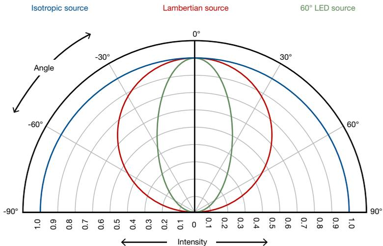
The cosine law therefore represents an ideal behavior, and the quality of sources, detectors and diffuse reflectors are usually measured by the degree of deviation from this ideal [1].
