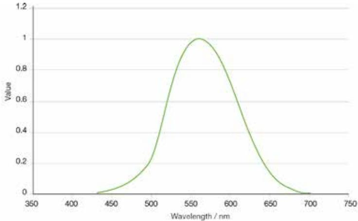
**Figure 1:** Diagram showing the  $V(\lambda)$  curve (human eye response function).
