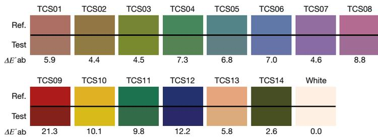
Figure 13 shows an example for rendering of Test Color Samples (TCS) by two sources. CIE Publication 13.3 [5] describes the recommended calculation of the CRI. Details of the calculation will be omitted here but essentially the method follows these steps:
