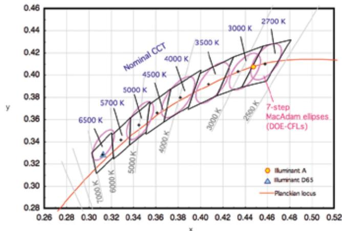
Figure 16 shows the Energy Star® binning limits for integral LED lamps. This principle of color binning is adopted from the American National Standard ANSI\_NEMA C78.377 “Specifications for the Chromaticity of Solid-State
