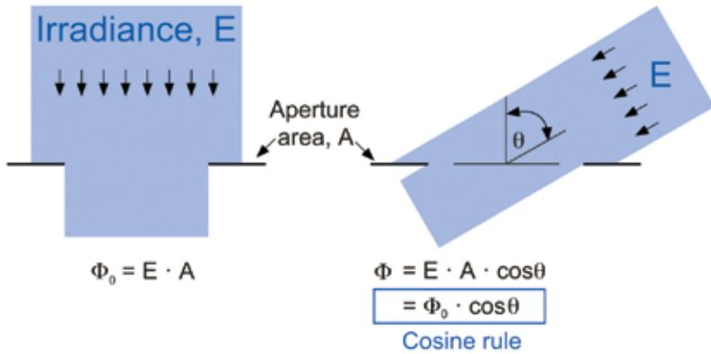
In order to correctly measure the irradiance at a plane, the detector must feature this cosine response so that light from all angles is weighted correctly. A source of radiance that includes a good cosine distribution is called a Lambertian source. A perfect diffuse reflector will scatter light so that the reflection is Lambertian (a cosine distribution) irrespective of the direction of illumination used.
