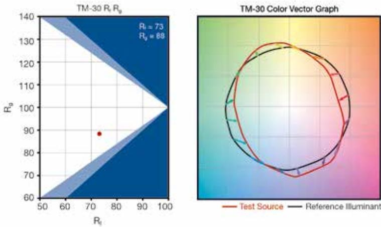
**Figure 18:** Gamut Index versus Fidelity Index with approximate limits for the combination of the two measures (left). The shaded areas are not achievable for practicable white light sources and for sources on the Planckian locus. Color Vector Graphic for a typical white light source (right). Tangential vectors to the reference circle indicate hue shifts. Vectors pointing inside/outside the reference circle indicate decreased/increased saturation for the specific color.
