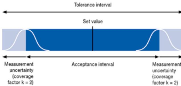
**Figure 15:** Relationship between set value, expanded measurement uncertainty, tolerance and acceptance interval. The definition of the tolerance interval does not take account of measurement uncertainty.
