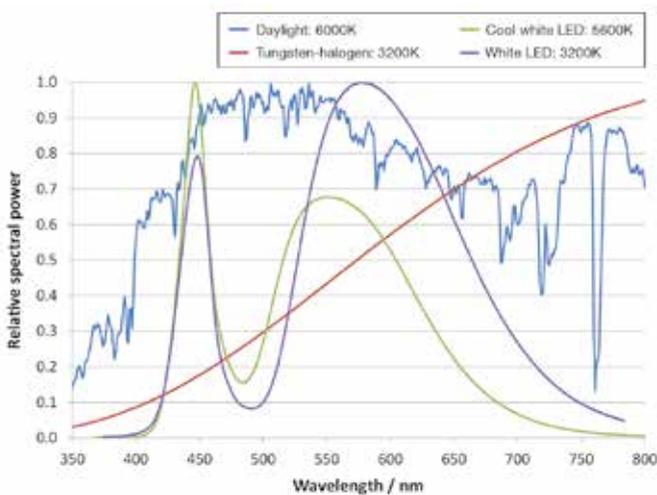
**Figure 12:** Examples of source spectra with their respective CCT.
