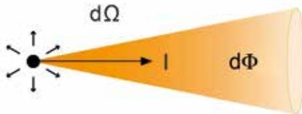
Radiant intensity  $I_e$  is defined as radiant power  $d\Phi_e$  emitted per unit solid angle  $d\Omega$  in a given direction (refer to Figure 3). It is expressed in watts per steradian [W sr<sup>-1</sup>].
