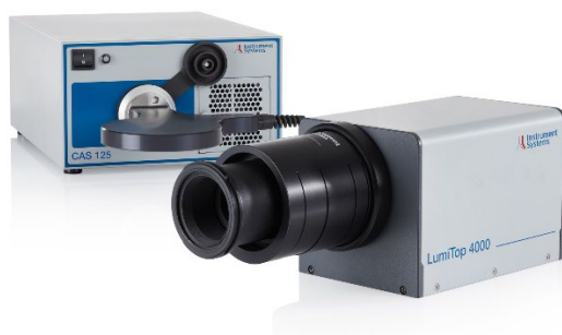
Figure: Compared to the single measurement of each LED of the wafer, the simultaneous measuring LumiTop system is orders of magnitude faster and still provides spatial and spectral information for each individual emitter.
