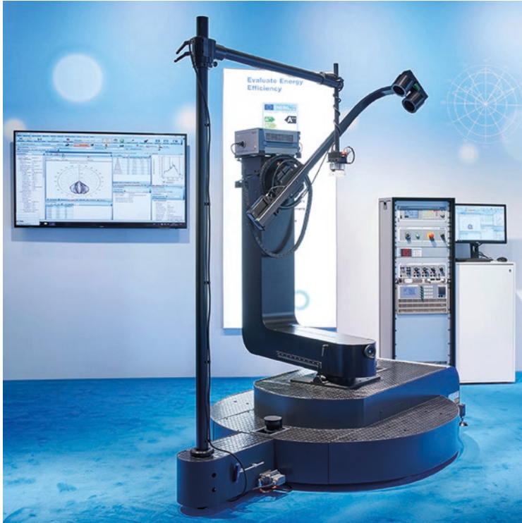
Figure: In order to precisely determine the radiation characteristics and luminous flux of an SSL source, angle-dependent properties are comprehensively characterized using an LGS goniometer system.
