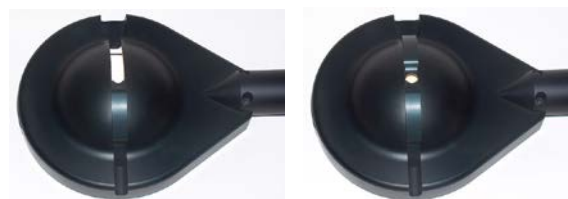
Figure 3: Gloss-trap slit partially closed (SCI/SPINC for microscope inclinations \geq 10^\circ ; left); gloss-trap slit closed (microscope inclination restricted to 0^\circ ; right).
