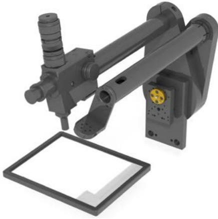
▲ Figure 19: PLS mounted at the reflective illumination arm of a DMS 803 / 505.
