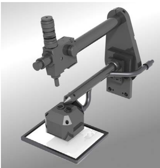
▲ Figure 7: SDR with measurement microscope and additional optics for modification of the focusing distance.
