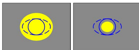
Figure 15: Measurement field (blue circle) overfilled: The illuminated area of the DUT (yellow) is larger than the measurement field (left). Measurement field (blue circle) underfilled: The illuminated area of the DUT (yellow) is smaller than the measurement field (right).
