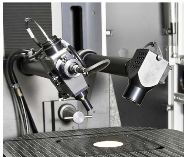
Figure 13: VADIS mounted at the reflective illumination arm of a DMS 803.
